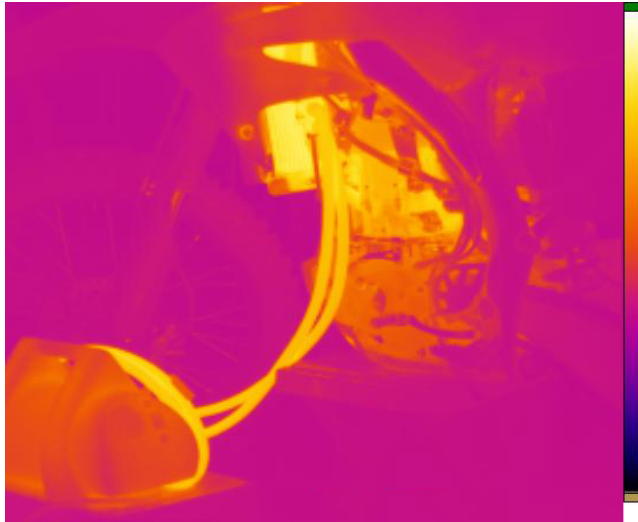
A thermal image of a preheater heating a single-cylinder engine. The vertical bar at right indicates the temperature gradient.
